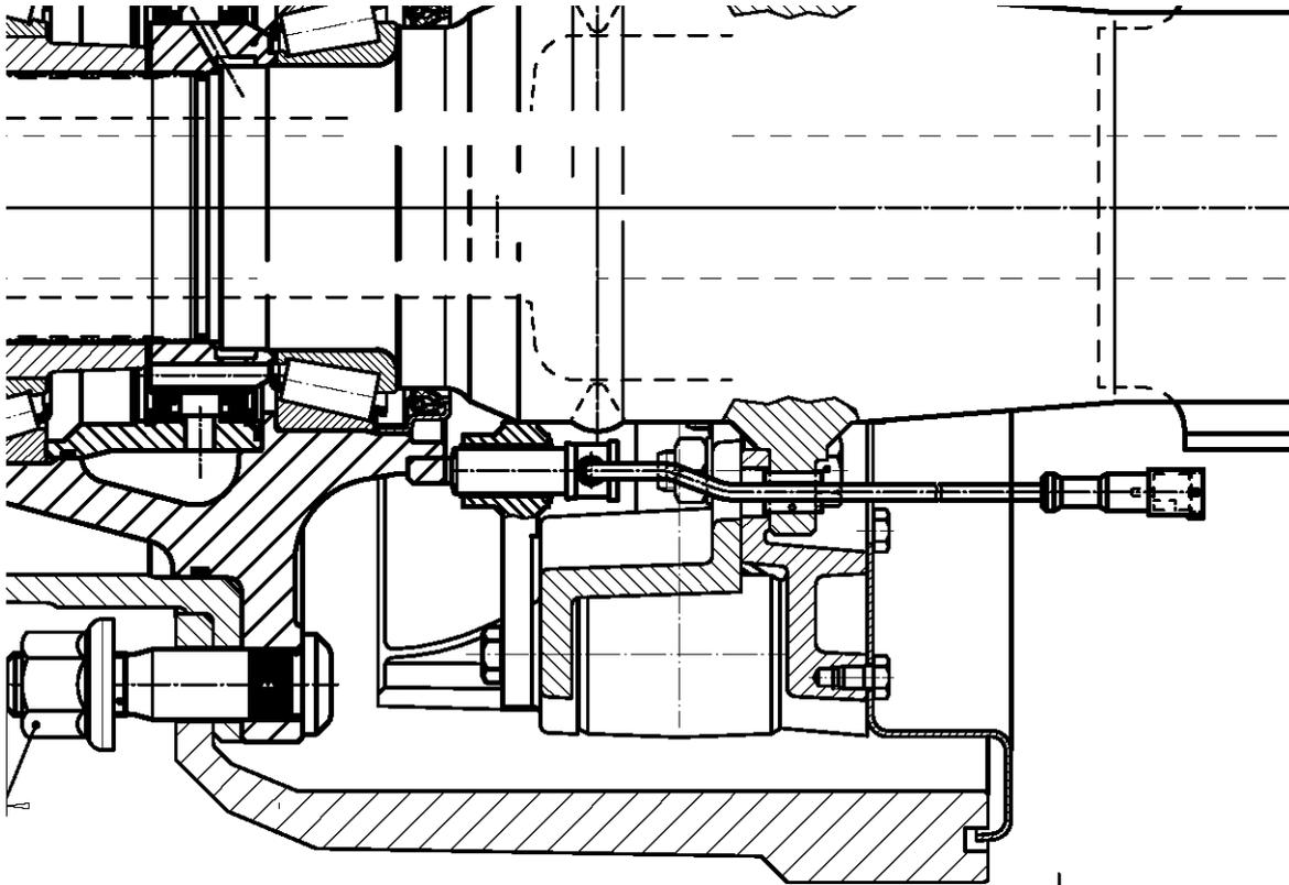
**Picture 2. Principle drawing of ABS sensor positioning and wire routing**
