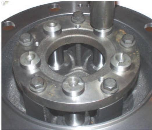
Picture 13. Installation of the planet gear shafts.
