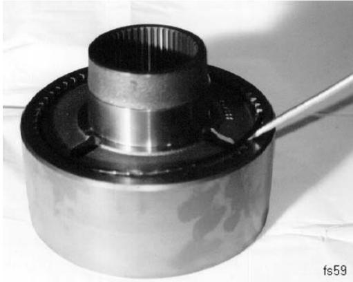
Remove the retaining ring. Remove the ring gear from the ring gear hub by tapping lightly with a soft metal hammer.
