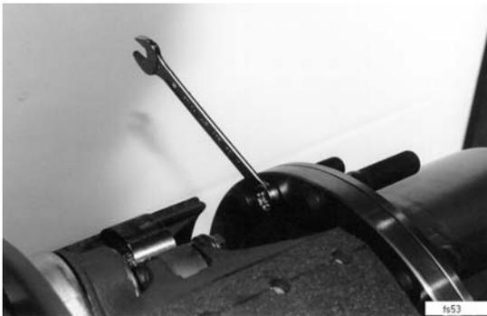
Picture 2. Unscrewing hub housing retaining screws.
