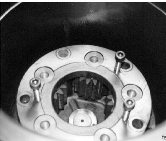
Picture 5. Using planet carrier cover pulling screws.
