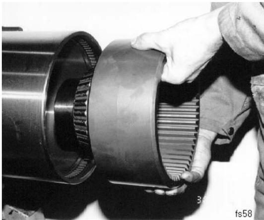
Picture 8. Removing the ring gear and the ring gear hub.
