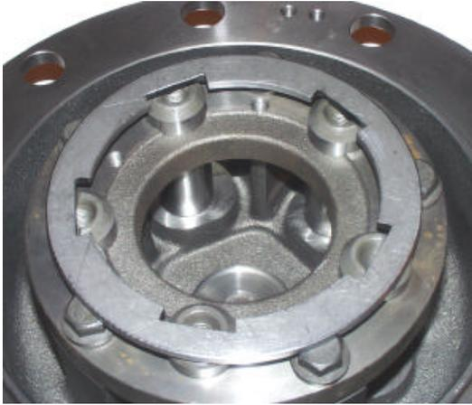
Picture 12. Positioning of the planet gear shafts
