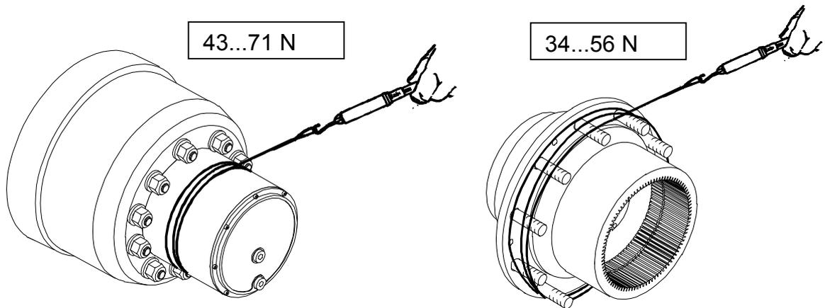
Picture 2. Rolling torque measurement with a spring scale from the wheel hub circumference.
