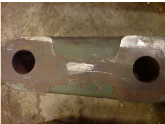
Picture 1. Faulty mounting surface in tie rod arm
